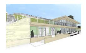
An accessible lift will be installed to connect the lower promenade with the first-floor level and greatly improve accessibility between the Upper Esplanade and Lower Promenade for wheelchair and pushchair users. Work is scheduled for completion by May 2025.
